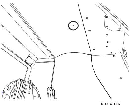
To access the (2) rear fixings, unlock and remove the upper access door.
