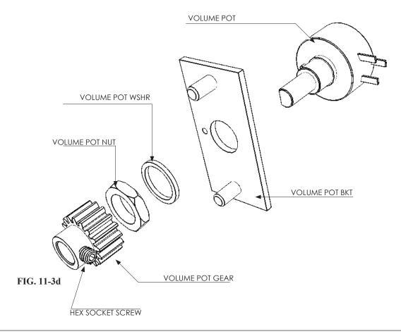
The wire connected to the volume pot will be reused. Use a tool such as a pair of snips or cutters to remove the old heatshrink tubes which cover the contacts.
