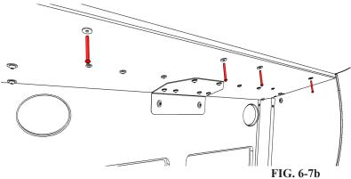
Secure the (4) M6 Fixings on top of the MONITOR CABINET in the orientation show in illustration (facing down into the cabinet).
