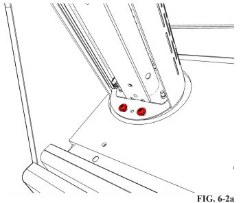
Have one person offer up the Exhaust Pipe and align with the fixing points shown.
