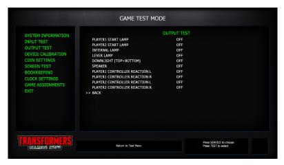
FIG. 6-18b OUTPUT TEST Screen
