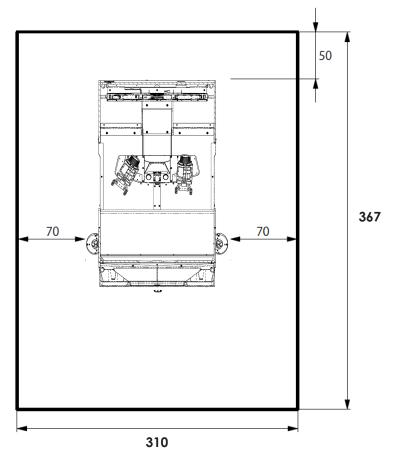
FIG. 2 Installation and operation area (cm)
