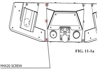
Remove the (5) Internal Hex screw which secure the Control Panel Cover.
