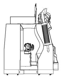
FIG. 7-1b Separate components when moving over a sloped or stepped area.
