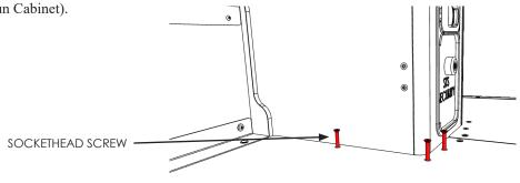
2 Secure the REAR SASH to the seat of the REAR CABINET using the (4) M4 fixings as shown.
