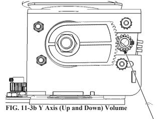
Position of Volume axis D cut face when controller pointing upper most postion.
