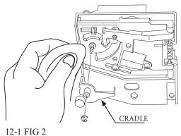
After wiping off as per previous step, further apply a dry cloth to completely dry the Coin Selector.
