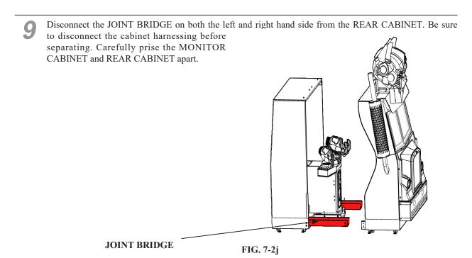
To reassemble, follow these steps in reverse order. Also refer to the Installation Guide within Section 6 of this manual. If the MONITOR CABINET is still too wide, remove the JOINT BRIDGE brackets and compress the gun cabinet (see Section 6 for details on how to compress/extend the gun cabinet).
