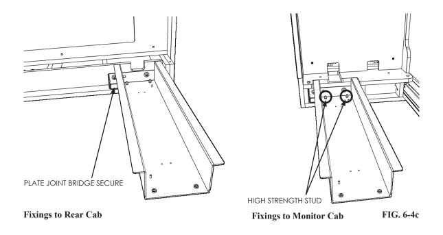
After securing the JOINT BRIDGE units, on the left hand side (JOINT BRIDGE L), feed the wiring harnesses through the JOINT BRIDGE L and connect to the REAR CABINET harnessing.
