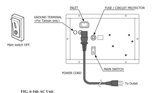
Fully insert the power cord connector on the side opposite the power plug into the AC unit inlet.
