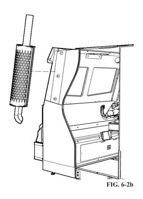
Using the (2) M8 fixings removed in Step 1, secure the Exhaust Pipe to the top of the REAR CABINET.
