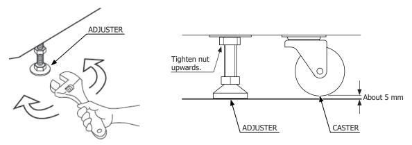
FIG. 6-13b Aligning the Adjusters
