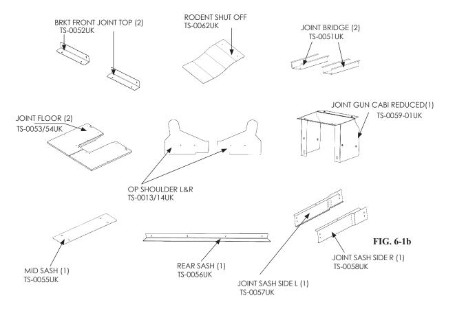
Below is a illustrated diagram of the where the previously listed components and brackets can be found after unpacking the cabinet.
