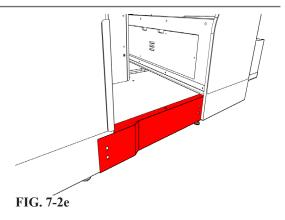
Remove the MID SASH bracket connecting the two floor panels.
