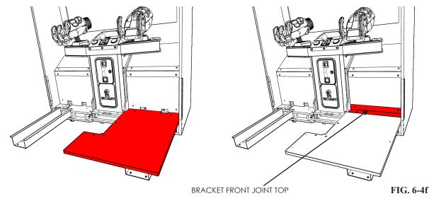
Extend the Gun Cabinet fully, ensuring that the fixing points are aligned with those of the RH Floor Panel.
