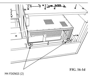
Lift and remove the Game board from the cabinet. The Game Bd is HEAVY so take care not to clash with other components when removing as this could cause component damage.
