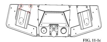
**5** Carefully slide the base plate out towards the front of the cabinet.
