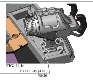
Lift the Control Unit directly upward and remove it. Be sure to feed the harnessing wires through when removing the Control Unit.
