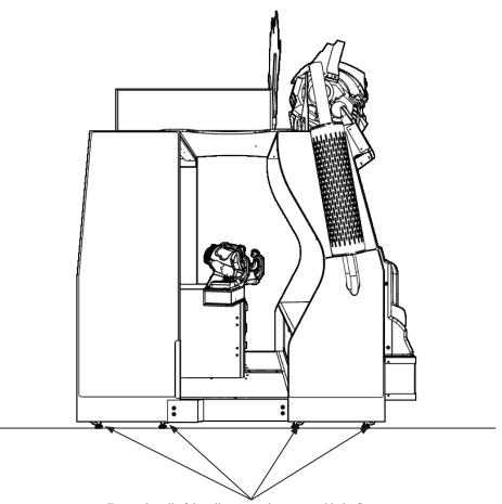
Ensure that all of the adjusters are in contact with the floor.
