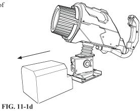
Remove the (4) M8 hex bolts from the base of the controller. Disconnect all harnesses.
