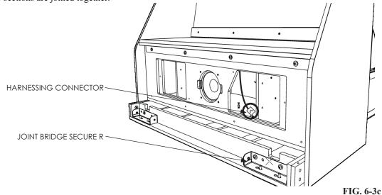
Secure the seat panel with the (4) M8 fixings shown and place the DOOR SEAT LOWER in place.
