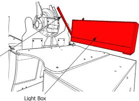
Remove the (8) M8 fixings that secure the roof panel to both sections of the cabinet and remove the roof panel.
