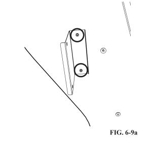
2 Secure the BRKT SUPPORT SHOULDER to the roof of the Rear Cabinet using the (2) M6 fixings. Note: these fixings are orientated "up", meaning they are secured from inside the cabinet facing up and out.
