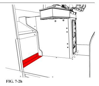
Remove both the left and right FLOOR PANELS. Disconnect the harnessing between the REAR and MONITOR CABINET.
