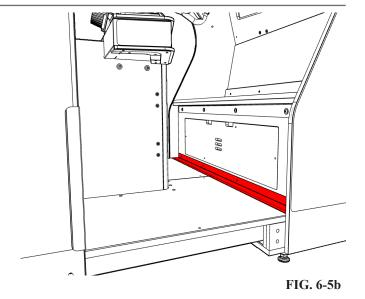
Secure the MID SASH using the (4) M4 fixings to secure the connection between the two FLOOR PANELS
