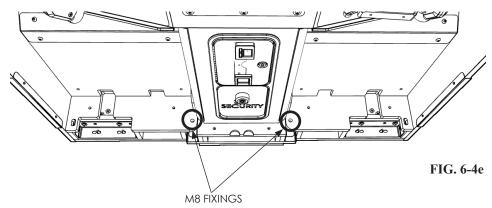
Place the RH Floor Panel into position and secure using the BRACKET FRONT JOINT TOP (this bracket is in situ and must be removed before placing the floor panel and then reapplied).
