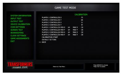
FIG. 9-6a CALIBRATION Screen
