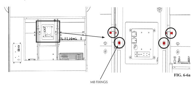
**9** Secure the (4) M8 fixings of the JOINT GUN CABI REDUCED
