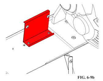
Remove the (2) highlighted M6 fixings.
